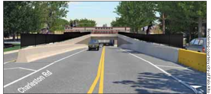
The Charleston Road underpass, which would keep the train tracks in their current alignment and reconfigure the roads at the rail crossing, is among the alternatives that the Palo Alto City Council is considering for grade separation.
