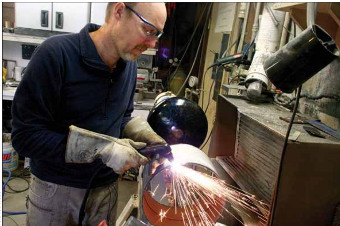
Above: As sparks fly, Steve "Spike" Finch uses a plasma cutter to saw the top off a propane tank, which he'll later turn into a Zem Tambour drum. Below: Finch shows how he takes two propane-tank tops to turn into a drum.
