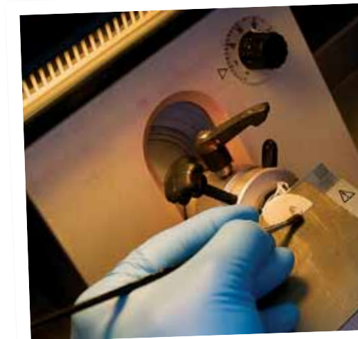
A technician prepares a five micron-thin frozen sample for Gladstone's microscopic examination.
